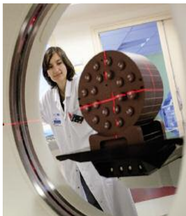
Quality control of a CT installation by a medical physicist at the Pitié Salpêtrière Hospital in Paris
