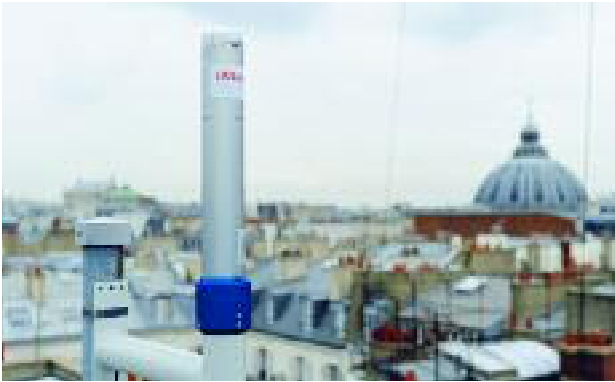
New-generation IRSN T  leray network monitor designed to monitor ambient gamma radiation in France, installed on the roof of the Navy headquarters in Paris.
